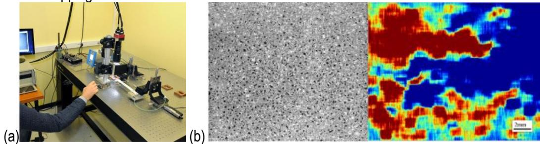
Figure 1 : (a) View of a tribometer with in situ visualization of contacts by fast camera. (a) In situ views of micro-contacts (black) in a rough PDMS/Glass interface and mapping of local micro-slipping events (in red) in the transient friction phase.
